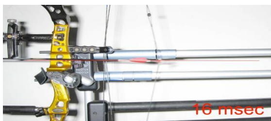
16 msec and the flex has changed and the arrow has started to lift off the rest.
